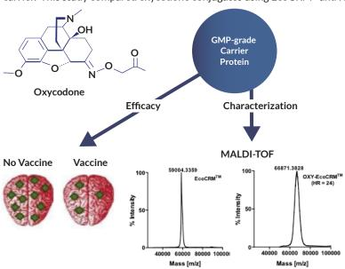
EcoCRM® was analyzed by MALDI-TOF before and after conjugation to the OXY hapten. A ratio of 24 haptens per  ${\sf CRM}_{197}$  was calculated from the MW difference. KLH conjugates were too large to be characterized by mass spec.
